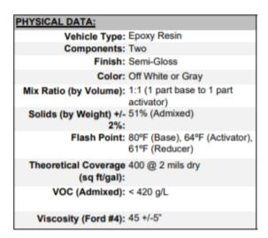
Note: The technical data sheet is reference the application and physical data of the primer. From "2-Part
