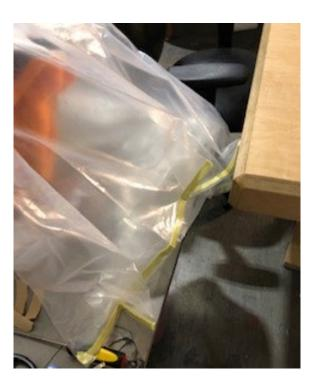
*Note:* The pleats in vacuum bagging are important to allow the bag more travel room than the width of the bag, especially for female molds with a hollow center like the once constructed. From Navarro-Luviano, 2022. Photograph.
