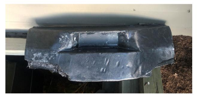
*Note:* The carbon fiber dash that a vacuum bagging method was attempted but failed. Navarro-Luviano, 2022. Photograph
