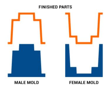
*Note:* How the composite tools of the dash were constructed and distinguished. From "Mold Construction Guide", n.d.. <u>https://www.fibreglast.com/product/mold-construction/Learning\_Center</u>.
