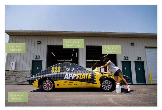
*Note:* Picture of R.O.S.E pointing to all the carbon fiber parts in the car. From Willoughby, 2021.
