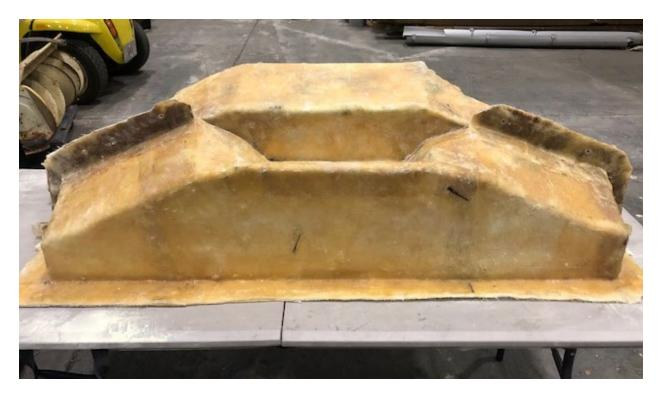
*Note:* With the two halves together one can clearly see how the flanges allow for easy assembly and disassembly of the mold. From Navarro-Luviano, 2022. Photograph.
