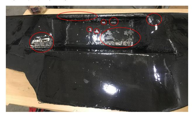
*Note:* The first carbon fiber dash is produced, but with many voids and unsatisfactory surface. From Navarro-Luviano, 2020. Photograph.
