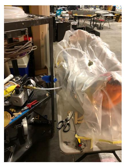
*Note:* In the image above a depiction of the vacuum bagging set up is shown. The connection is the reduces on of just having the hose go from the vacuum pump to the vacuum valve on the dash. From Navarro-Luviano, 2022. Photograph.
