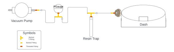
*Note:* This schematic of the setup is to illustrate how everything was originally connected before it had to be reduced to just a connection from the pump to the vacuum valve on the dash. From Navarro-Luviano, 2022. LucidCharts.
