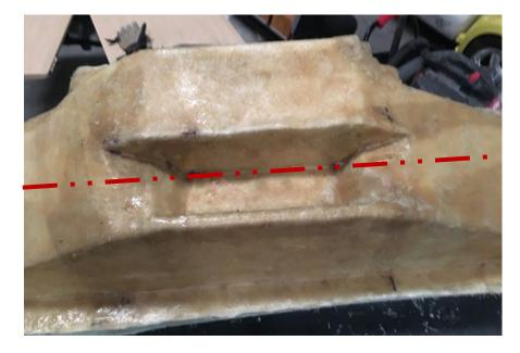
Line marking where the piece had to be cut to remove the finished fiberglass part.
